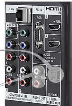
Typical TV Back-Panel Connectors
